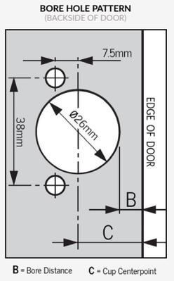
**BORE HOLE PATTERN (BACKSIDE OF DOOR)**
